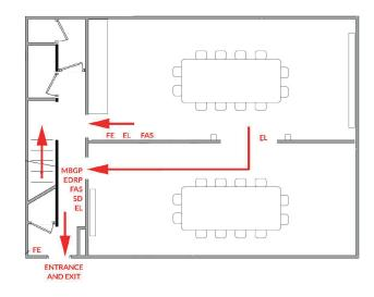
FAS - Fire Alarm Sounders SD - Smoke Detectors EL - Emergency Lighting FE - Fire Extinguishers EDRP - Emergency Door Release Point FAS - Fire Alarm Sounders MBGP - Manual Break Glass Point
